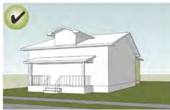
One story attached addition Addition is set back behind the original building.
