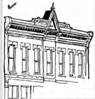
Reconstruct a missing cornice when historic evidence is available.
